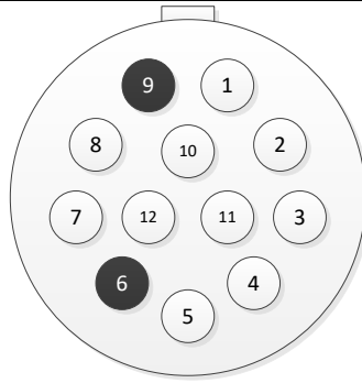
Figure 5: GPIO Interface Connector Pin Out (P201)
