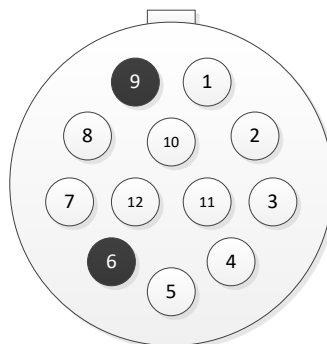
Figure 5: GPIO Interface Connector Pin Out (P201)
