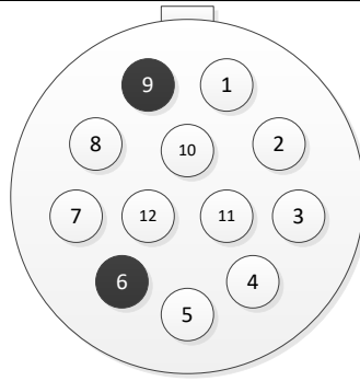
Figure 5: GPIO Interface Connector Pin Out (P201)
