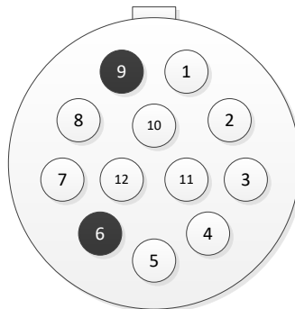
Figure 5: GPIO Interface Connector Pin Out (P201)
