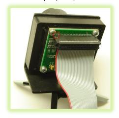
3) Connect the supplied Null Modem serial cable and 10pin to the header near the power input. Configure your PC serial port application with: 115200 baud rate, 8 data bits, no parity, 1 stop bit and no flow control.
