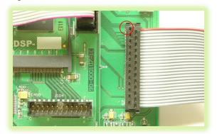
2) Connect the other end of the 26-Pin cable to the Vision Camera as shown with the red stripe towards the top left. Attach the tripod (varies) to the camera as well.
