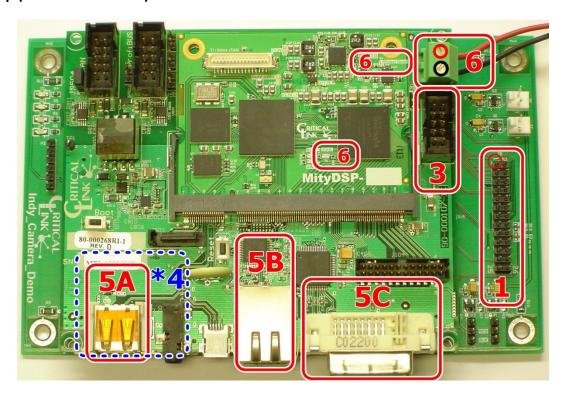
\*4: SD Card is on the bottom side of the board
