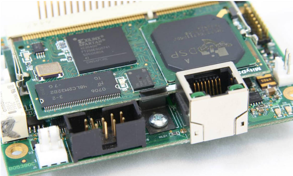
Figure 6: Photo of MityDSP held in place by Metal Clip
