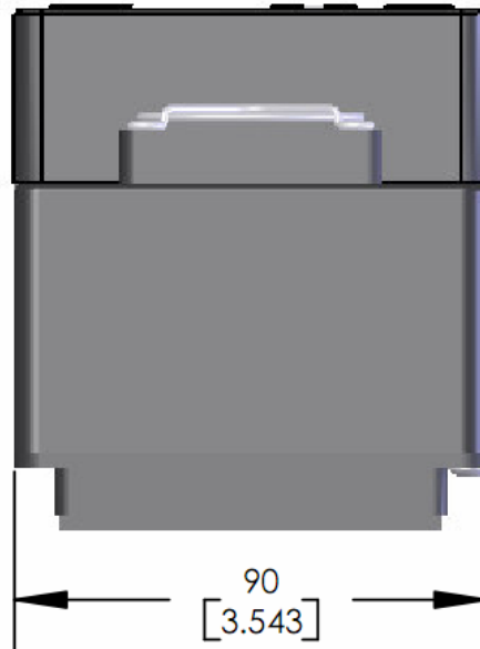
Figure 6: Standard Body (Type A) with Rectangular Flange (Type A) - Top View
